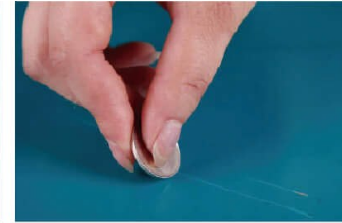
划刻硬度也称为耐划伤试验 Scribing hardness also known as scratch hardness test
